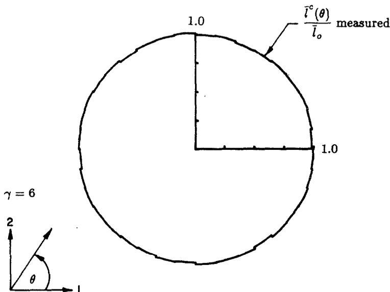
Fig. 4. Normalized distribution of contact lengths for 1000 disc assembly.
