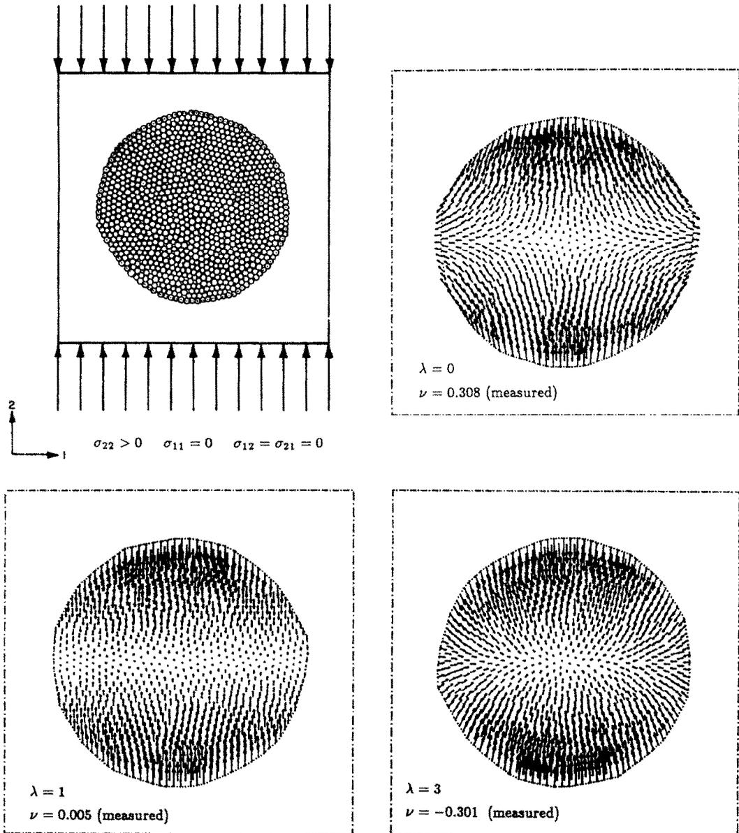
Fig. 7. Displacement fields for disc centres from biaxial compression tests with variable stiffness ratio  $\lambda$ .
