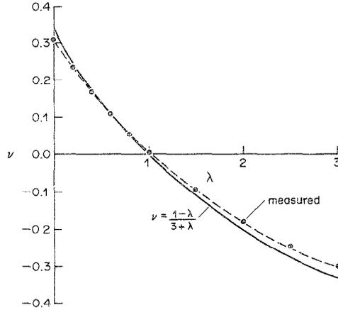
Fig. 8. Comparison of measured and theoretical values of Poisson's ratio  $\nu$  against stiffness ratio  $\lambda$ .
