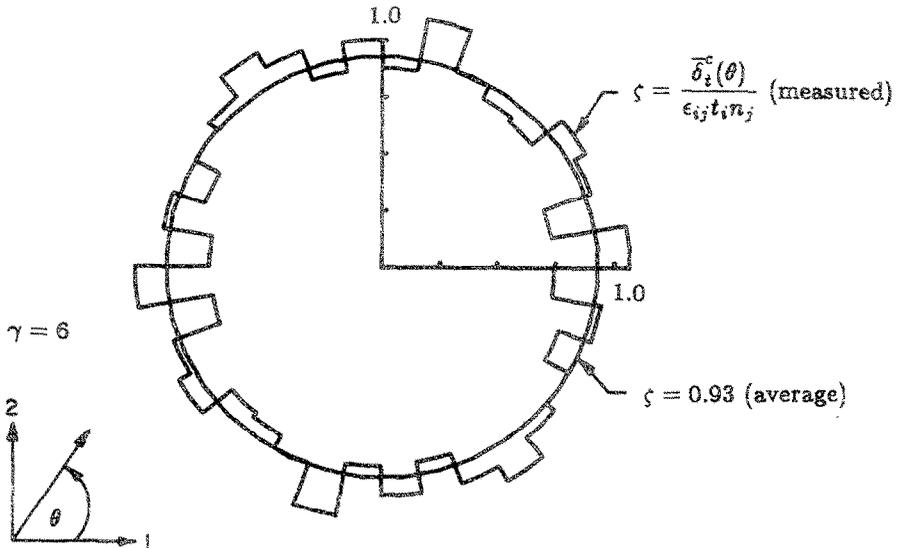
Fig. 5b. Coefficient  $\zeta$  from distribution of average tangential contact displacements  $\overline{\delta_t^c(\theta)}$ .
