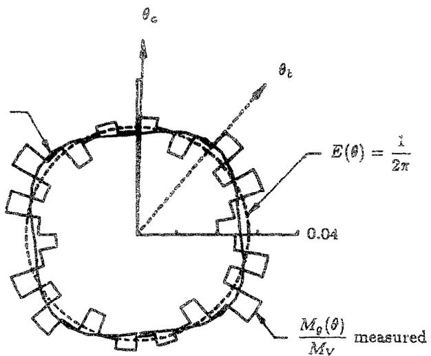
Fig. 3. Normalized distribution of contact orientations for 1000 disc assembly.
