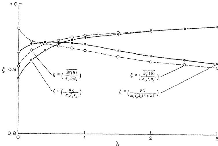
Fig. 6. Coefficient  $\zeta$  versus contact stiffness ratio  $\lambda$ .
