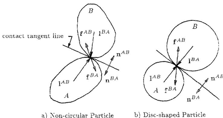
Fig. 1. Contact normals, contact vectors and contact forces.
